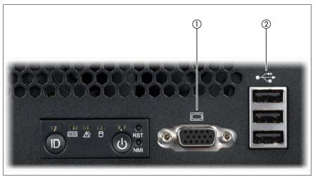
Figure 8: Connectors on the front
